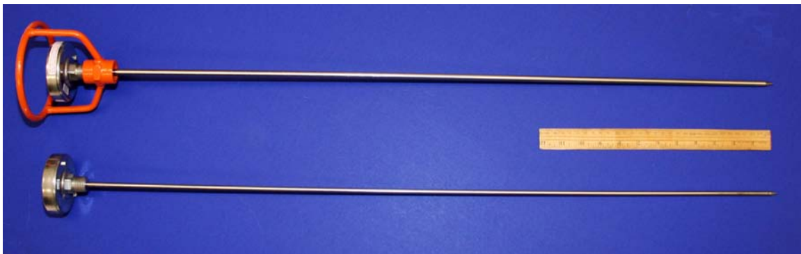
Figure 4. Compost thermometers are 3 to 4 feet long.
