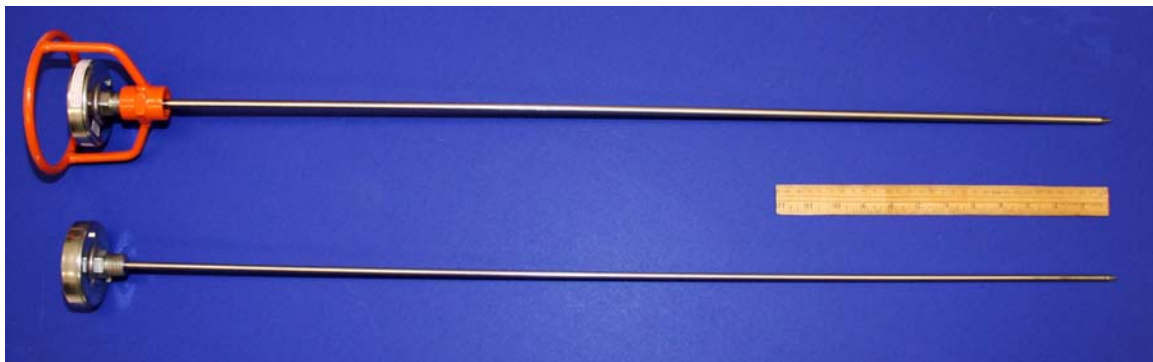
Figure 4. Compost thermometers are 3 to 4 feet long.
