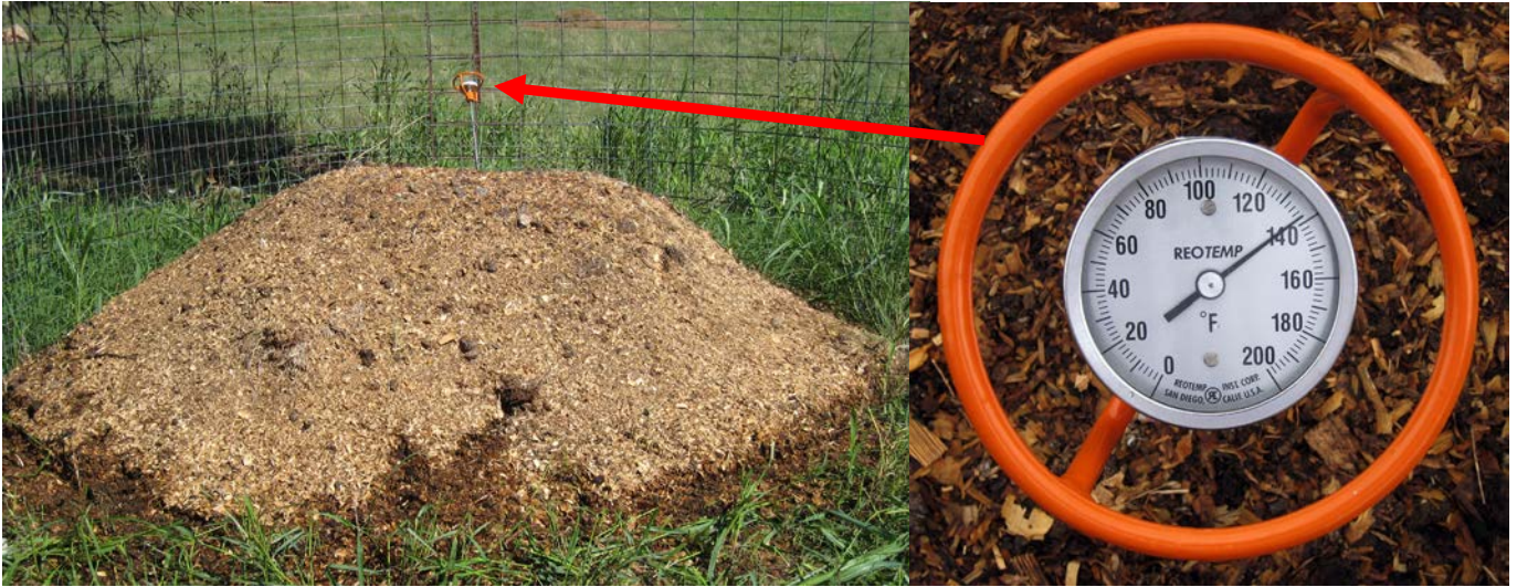
Figure 5. Compost thermometers should measure core temperature. Temperatures over 131° F kill most pathogens.
