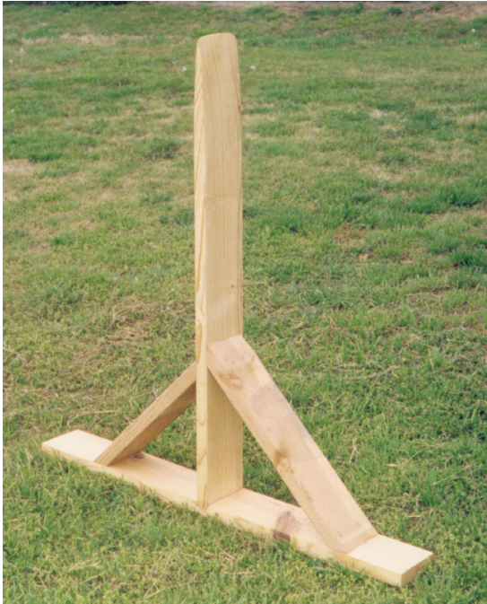
A staking beam looks like an inverted “T” with the top sanded to a blunt point (left). To soften the skin, pull it back and forth over the point of the beam (right).
