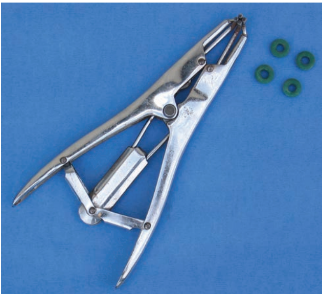
Elastrator with rubber bands.
