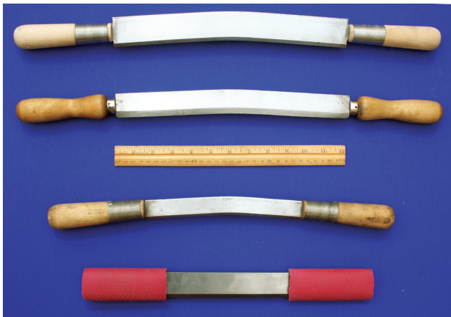
Different styles and sizes of fleshing knives (above). To flesh a hide, drape it over the fleshing beam with the tail nearest you. Lean into the beam to hold skin and scrape off all meat, fat, and membrane.
