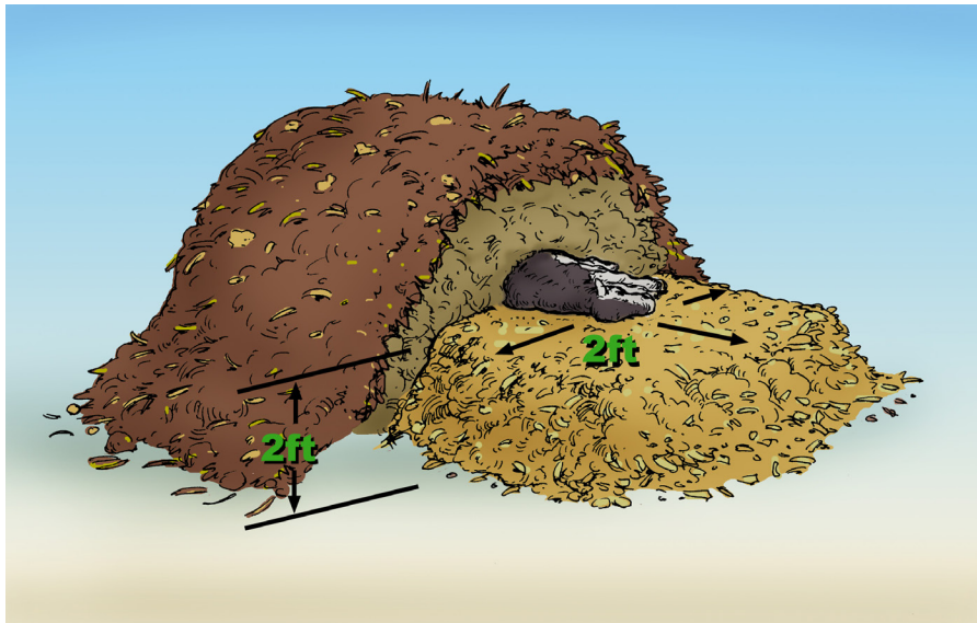
Make the base large enough to allow for a 2-foot clearance around the carcass.
