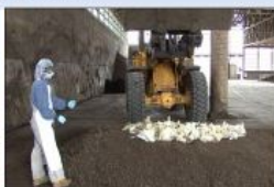
Static pile construction during a disease outbreak.
